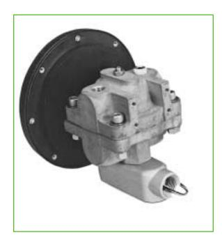
The Model 130 is available in Aluminum, Brass and 316SS bodies only with one or two hermetically sealed reed switches for low and/or high limit alarm. These CSA listed switches are single-pole, double-throw, and may be connected to open or close on rising or falling pressure.
